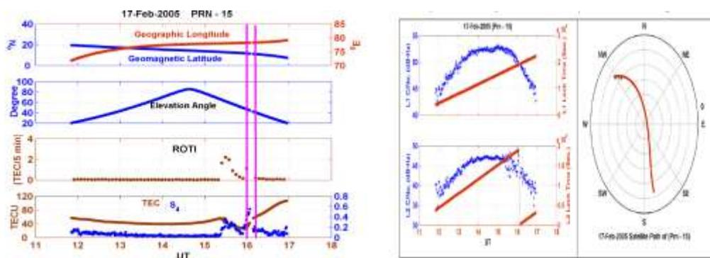
Figure: TEC depletions and loss of lock event observed by GPS receiver
