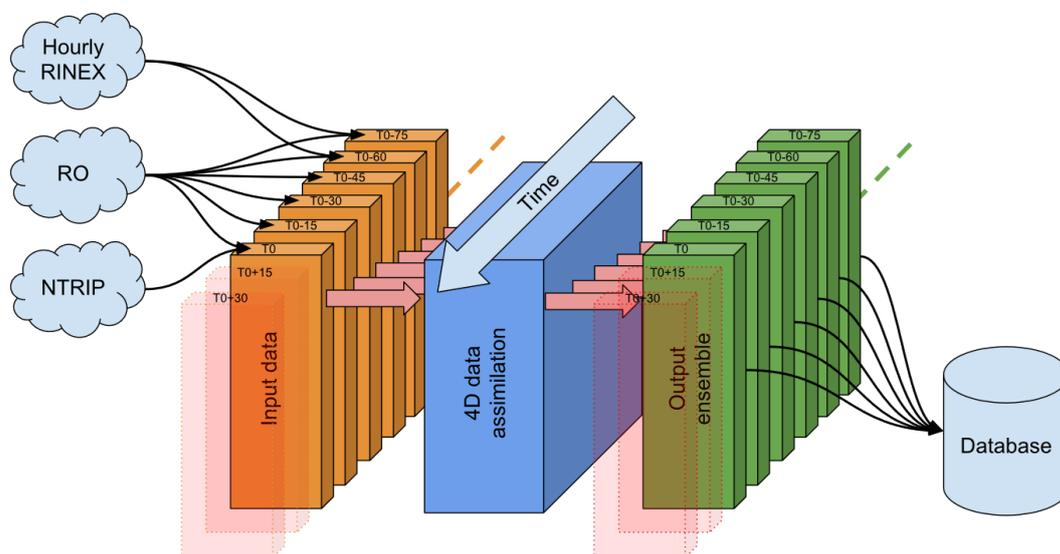
Figure 2. Cartoon showing how data with different latencies is packaged and used to drive the 4D data assimilation model
